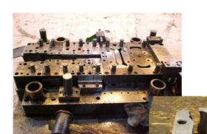
TOOLOX 44, nitrided Blanking of 3.8 mm 270 MPa sheet
