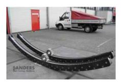
Curved gear rack for the Red Bridge draw bridge manufactured by SANDERS, the Netherlands.
