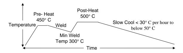
Prep the surface by filing or grinding out and cracks of loose debris. Pre-heat the part to be welded to 450 degrees Celsius (840 degrees Fahrenheit). Weld the part without letting it drop below 300 degrees Celsius (575 degrees Fahrenheit). Weld at as low as possible power setting and avoid weaving.
